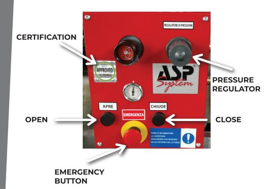
The system can fully or partially close the pit quickly and safely.
